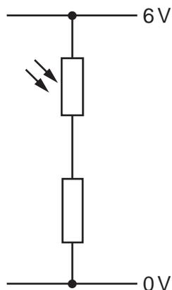
When brighter light falls on the light-dependent resistor (LDR), its resistance changes.
