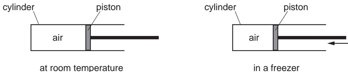
As the air cools, the piston moves to the left as shown.
